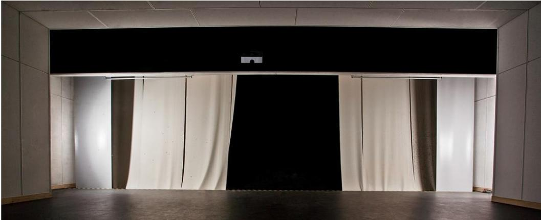
For use as a pure reflection medium, we recommend a thickness of 1.6mm. At this thickness, the **RUTEC** reflection tarpaulin also forms limited splinter protection that is suitable as an additional protection particularly for "soft" projectile capture devices. In a stronger design, **RUTEC** R1267 can be used as a reflection medium for hard projectile catching devices and complete splinter protection.
